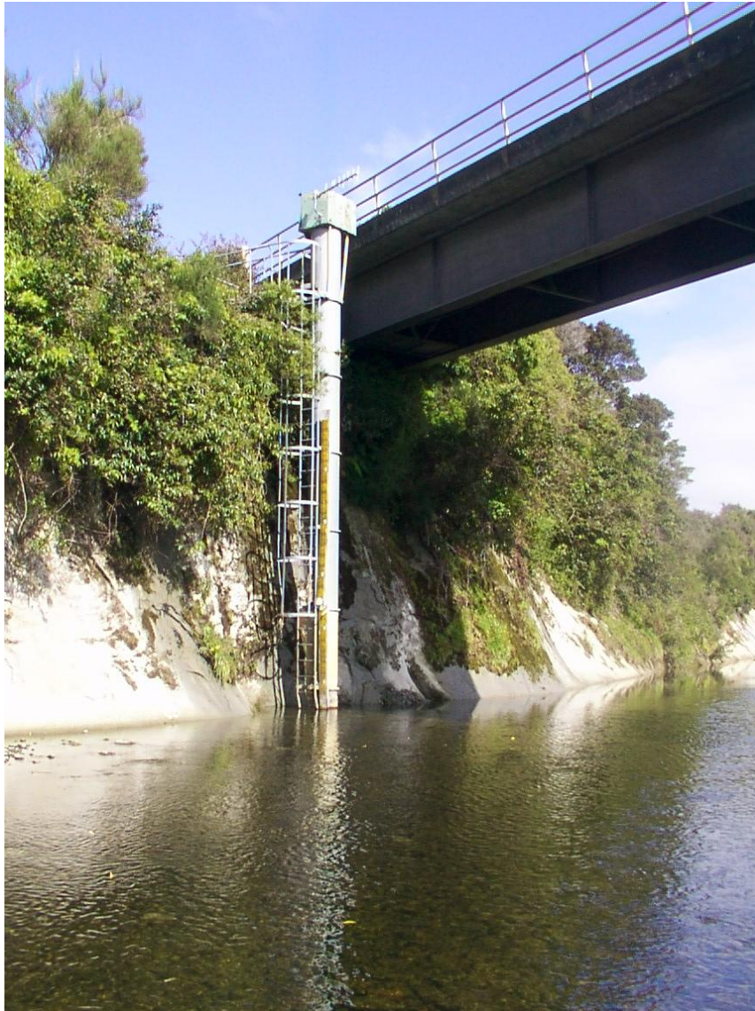
Figure 10 – Stilling well with multiple sections and housing.
