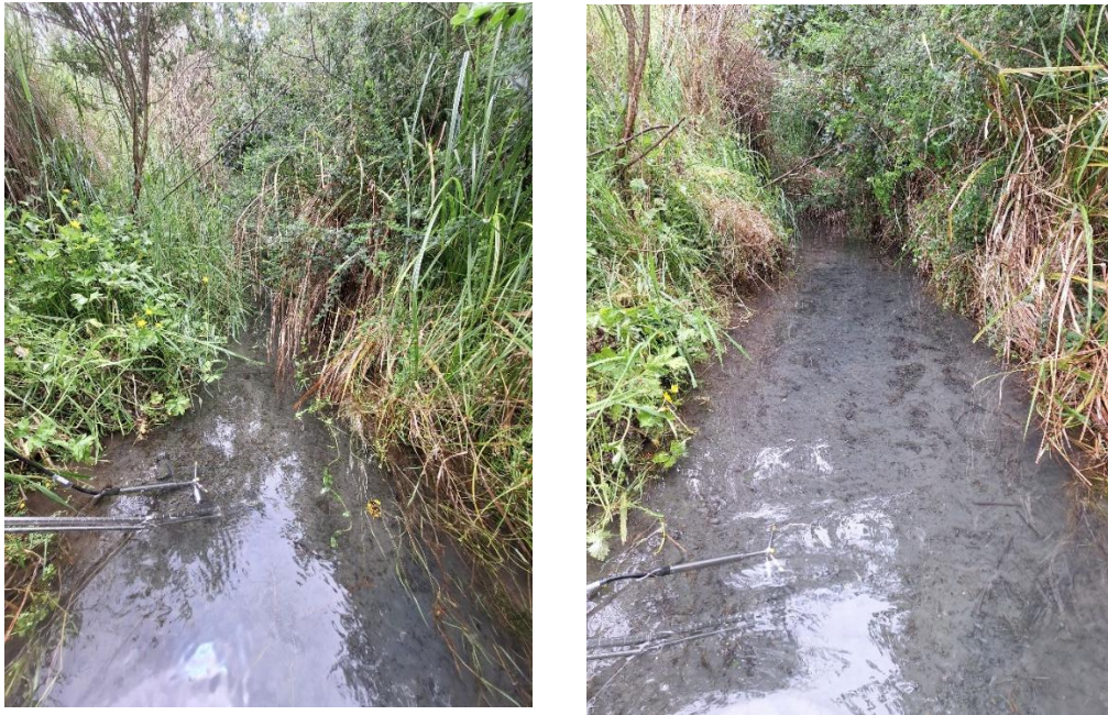
Figure 21 The left image shows a site with excessive bankside/surface vegetation in the flow. The stream was 1m wide and vegetation extended into the flow approximately 0.3m from the true left bank and 0.2m from the right for the entire length (3m) of the reach. This equates to 50% coverage and a site score of two (QC400). The right image shows the channel after vegetation clearance. This site now meets the requirements for QC600. However, being 0.3m deep, any submerged obstructions would need to be greater than 6m upstream.
