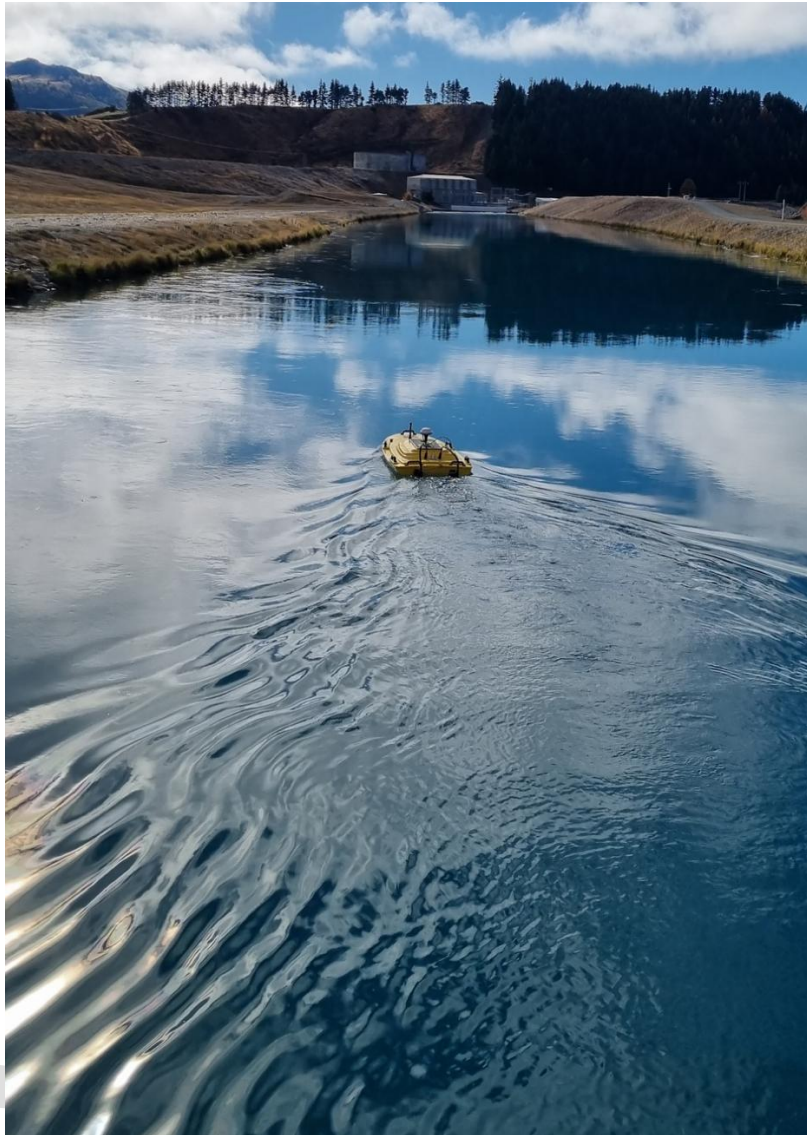
Figure 3 - Very good gauging cross-section where flow should be close to laminar
