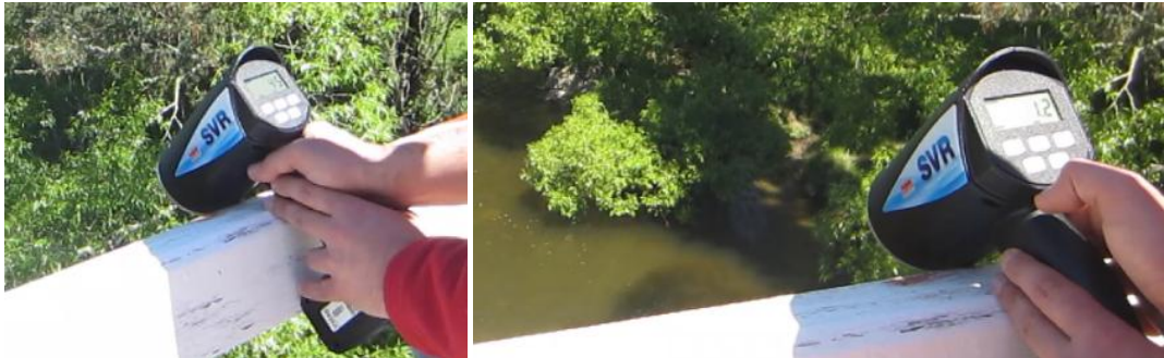
Figure H4: Shows a radar gun at 45 degree vertical angle (LHS) and velocity reading of 1.2m/s (RHS)
