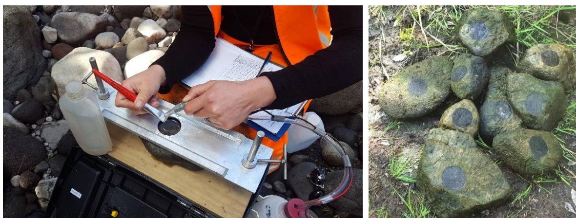
Figure 1 - A vacuum pump system (left) and rocks from which periphyton has been removed
