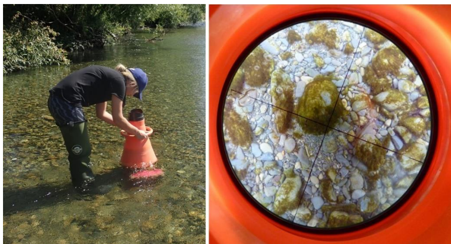
Figure 7 – Demonstrating the correct technique for use of an underwater viewer to estimate streambed cover (left) and the streambed as seen from looking down the viewer
