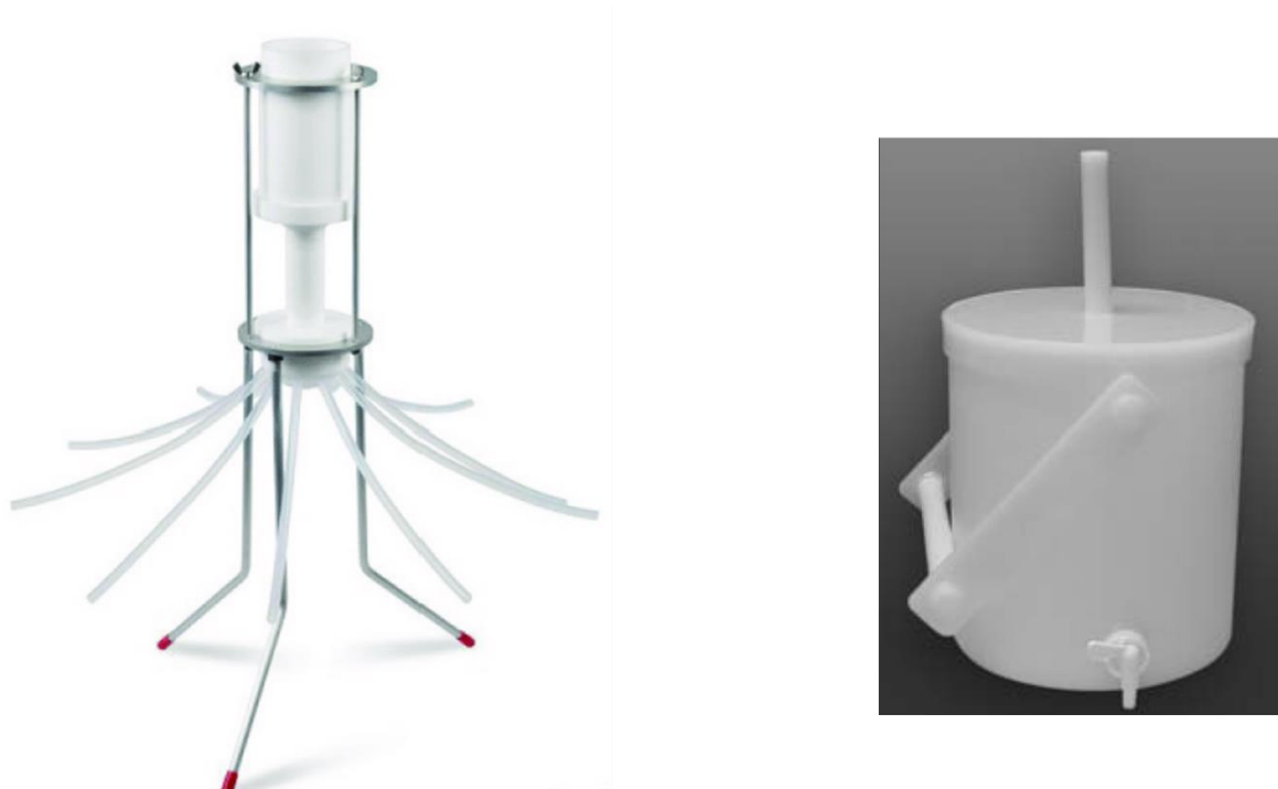
Figure 14-1 Sample splitters for reducing sediment mass for particle size analysis. Left: cone splitter (the original sample drains into multiple outlet pipes). Right: churn splitter (a sub-sample is drawn off via the spigot while the piston agitates and mixes the original sample).
