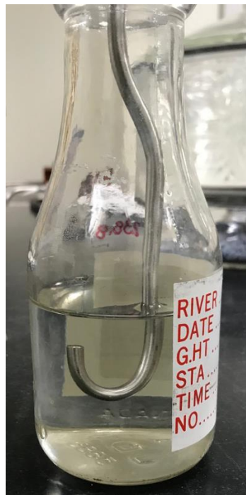
Figure 13-1 – J-tube (shown inside a glass sample bottle), used for decanting surplus clear water from a settled sample prior to evaporation when using ASTM D3977-37 Method A for SSC analysis. Photo courtesy of Stephen Low, USGS.
