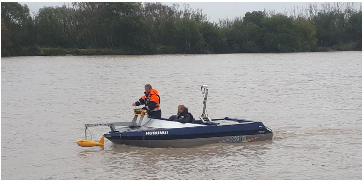
Figure 2-1 – A 48-kg US P-61 point sampler deployed from a jetboat using a bow-boom and gauging reel.
