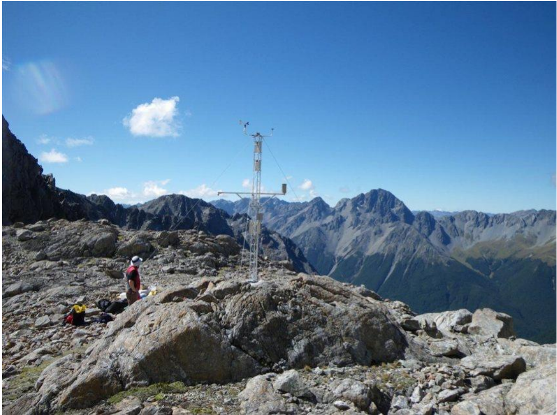
Figure 13 – Example of a 6-m lattice mast
