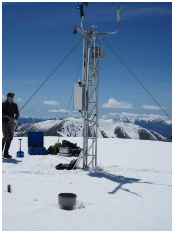
Figure 12– Example of a 3-m lattice mast
