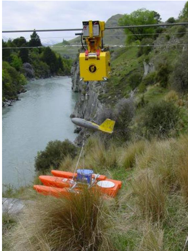
Figure 9 – Flow gauging using a ‘Hornet’ motorised slack-line system retrofitted to a manned cableway
