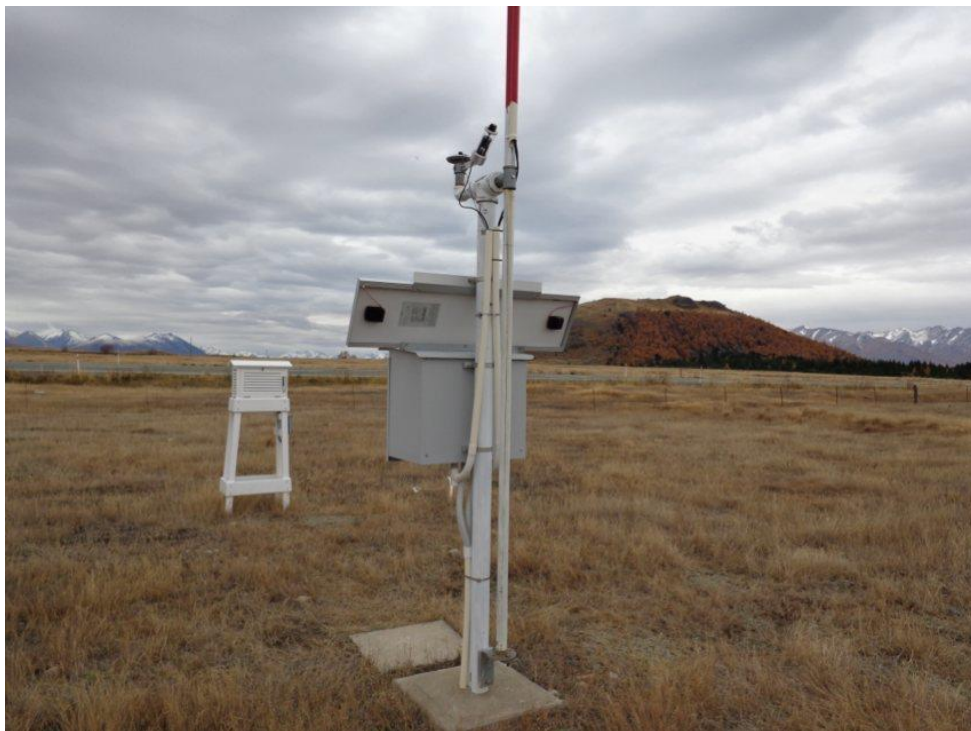
Figure 11 – Example of a 6-m tilting mast
