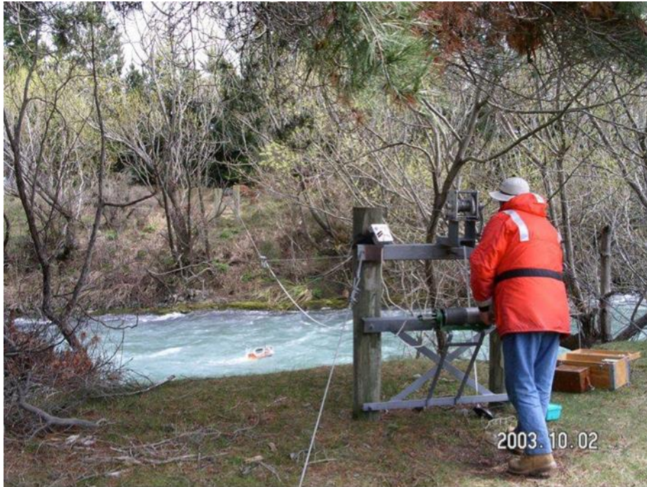
Figure 8 – Flow gauging from a manual winch slack-line cableway
