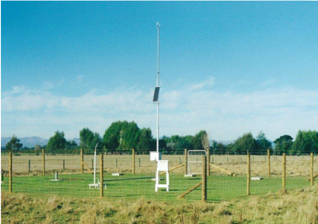
Figure 10 – Example of a 10-m tilting mast
